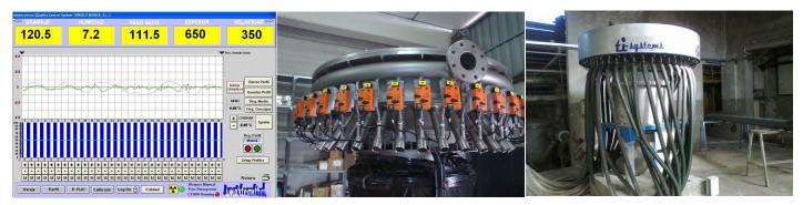
Radial Distributor with Intelligent Valves for Dilution Control. Basis Weight CD Control Systems adaptable to the most popular HeadBoxes. Also it's possible to make the control with Electronic Motors installed on the HeadBox lip. These options depends of the machine and also of customers requirements. Moisture CD Control Systems with Steam Boxes, Water Spray Systems or Infrared Drying Systems.
